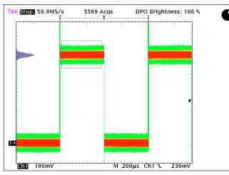
Figure 2. Histogram of noise on a square wave.
