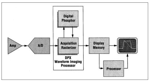
Figure 1. Tektronix DPO Architecture.
