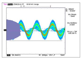
Figure 3. 1.85 GHz carrier and amplitude distribution of CDMA forward link, pilot only.
