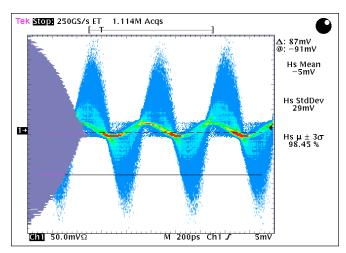
Figure 4. 1.85 GHz carrier and amplitude distribution, CDMA forward link. Walsh codes 0, 1, 8, 16, 24, 32, 40, 48, 56 at power levels per IS-97 recommendation.
