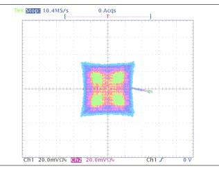
Figure 6. Unmodulated transient in demodulated CDMA forward link signal.
