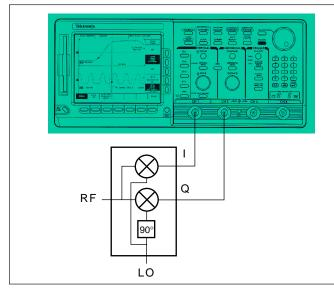
Figure 5. RF demodulation for live IQ displays.
