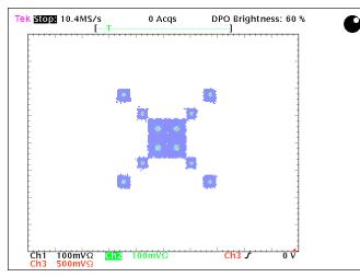
Figure 8. XYZ display of CDMA Forward Link.
